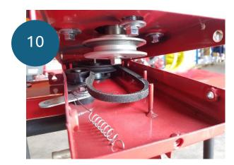
With the belt in place, lower the engine pully into the belt centre.
