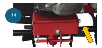
Put the inspection front plate back on and install the 2 side and front 10mm bolt.
