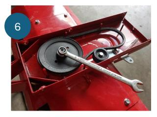
Remove the pully 13mm nut and washer.
