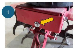
Remove the 10mm bolt from the inspection plate
