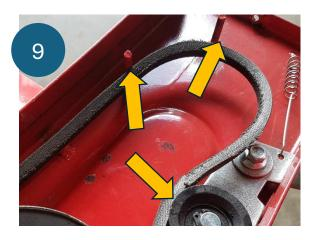
Pins and tensioner pully hold the belt in place.
