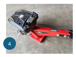
Lift engine and control arm to one side.
