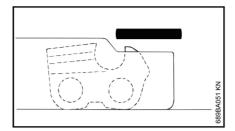
File down the depth gauge until it is level with the filing gauge.
