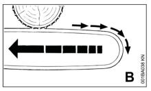
Pushback occurs when the chain on the top of the bar is suddenly stopped when it is pinched, caught or encounters a foreign object in the wood. The reaction of the chain may drive the saw rapidly straight back toward the operator and may cause loss of saw control. Pushback frequently occurs when the top of the bar is used for cutting.
