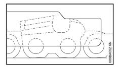
Place the filing gauge on the chain – the highest point of the depth gauge must be level with the filing gauge.
