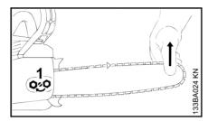
Retensioning during cutting work:
