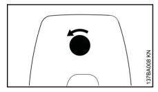
Turn the knob above the rear handle in the direction of the arrow and remove the carburetor box cover
