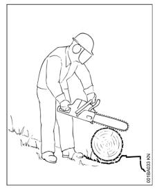
Bucking is cutting a log into sections.
