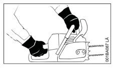
Your right hand should grip the rear handle. This also applies to left-handers. With your hands in this position, you can best oppose and absorb the push, pull and kickback forces of your saw without losing control (see section on reactive forces).
