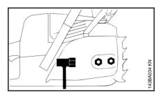
Unscrew the nuts and take off the chain sprocket cover.
