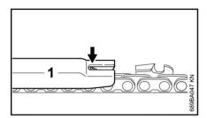
Place a filing gauge (1) that matches the chain pitch on the chain and press it against the cutter
