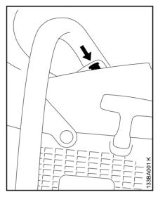
Press the button, the decompression valve will be opened
