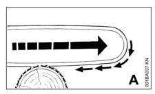
Pull-in occurs when the chain on the bottom of the bar is suddenly stopped when it is pinched, caught or encounters a foreign object in the wood. The reaction of the chain pulls the saw forward and may cause the operator to lose control.
