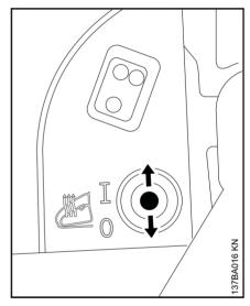
To switch on, set switch to I and to switch off, return switch to the 0 position
