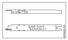
Use a filing gauge (special accessory, see table "Sharpening Tools"). This is a universal tool for checking the filing and side plate angles, depth gauge setting, cutter length and groove depth. It also cleans the guide bar groove and oil inlet holes.
