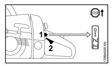
Press the throttle trigger lockout and blip the throttle trigger (2); the Master Control lever (1) jumps to the operating position I and the engine begins to idle
