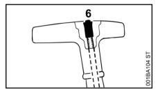
Press the remaining rope into the handle until the nippel (6) is flush with the handle
