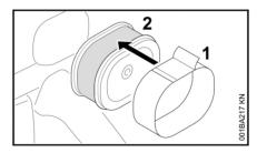
• Fit the felt prefilter (1) over the HD filter (2), note installation position
