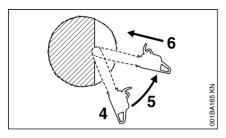
The plunge cut is made with the guide bar nose. Begin the plunge cut by applying the lower portion of the guide bar nose to the tree at an angle. Cut until the depth of the kerf is about the same as the width of the guide bar. Next, align the saw in the direction in which the recess is to be cut.
