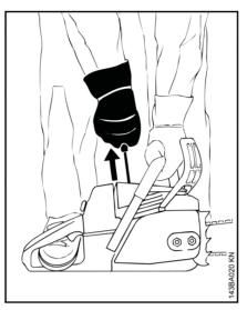
with the right hand, pull the starter grip slowly until you feel it engage and then give it a brisk strong pull simultaneously press down on the handlebar – do not pull the starter rope out all the way - risk of breakage! Do not let the starter grip snap back - guide it slowly back into the housing so that it can rewind properly
