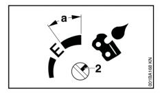
The oil pump with increased delivery rate can be identified by the groove (2) in the adjusting screw.
