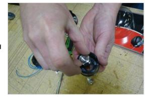
8. Reassemble the trimmer head by replacing parts in the reverse order that you removed them. These Speed-Heads are conveniently designed so that they can not be reassembled incorrectly. The design simply will not allow the two sides to close unless all the parts are installed properly.
