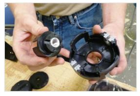
6. Press the thread adapter out with a hammer
