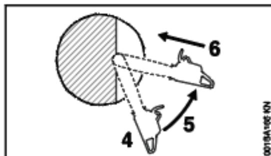
The plunge cut is made with the guide bar nose. Begin the plunge cut by applying the lower portion of the guide bar nose to the tree at an angle. Cut until the depth of the kerf is about the same as the width of the guide bar. Next, align the saw in the direction in which the recess is to be cut.
