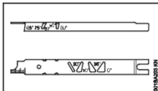
Use a filing gauge (special accessory, see table "Sharpening Tools"). This is a universal tool for checking the filing and side plate angles, depth gauge setting, cutter length and groove depth. It also cleans the guide bar groove and oil inlet holes.
