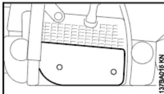
Under extreme winter conditions (temperatures below +14 °F (-10 °C), powdered or drifting snow), it is recommended to mount the cover plate (special accessory) on the fan housing.
