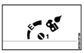
The oil delivery rate can be adjusted as needed using the adjusting screw (1) (on the bottom of the machine).
