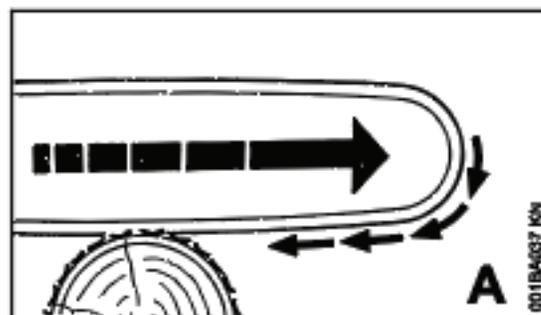
Pull-in occurs when the chain on the bottom of the bar is suddenly stopped when it is pinched, caught or encounters a foreign object in the wood. The reaction of the chain pulls the saw forward and may cause the operator to lose control.
