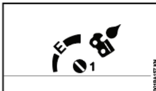
The oil delivery rate can be adjusted as needed using the adjusting screw (1) (on the bottom of the machine).
