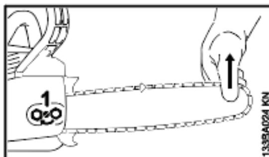
Retensioning during cutting work:
