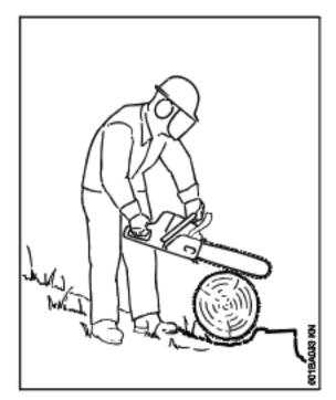
Bucking is cutting a log into sections.
