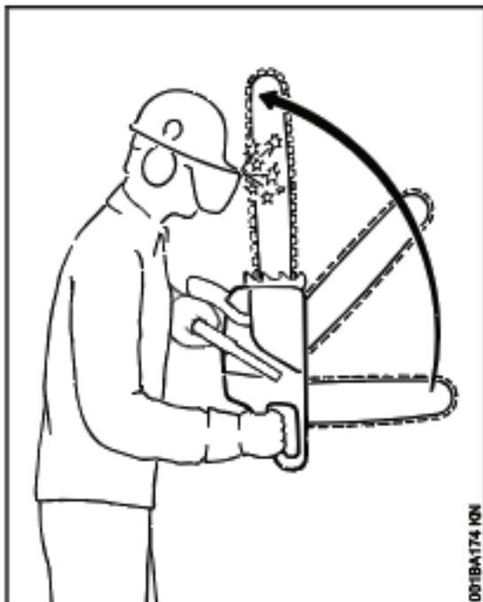
All chain saws are equipped with a Quickstop chain brake which can be activated by inertia. If the forces of an occurring kickback are sufficiently high, the hand guard is accelerated towards the bar nose even without hand contact. See the chapter entitled "Chain Brake" of your instruction manual.
