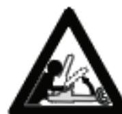
Kickback may occur when the moving saw chain near the upper quadrant of the bar nose contacts a solid object or is pinched.
