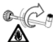
Unit vibrations can cause an improperly tightened fuel filler cap to loosen or come off and spill quantities of fuel. In order to reduce the risk
