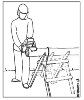
When cutting small logs, place log through "V"-shaped supports on top of a sawhorse. Never permit another person to hold the log. Never hold the log with your leg or foot.
