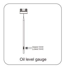
Fill to the upper limit (marked with "H") of the dipstick with the recommended oil if the oil level is low.
