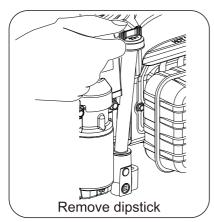
Remove the dipstick again and check oil level. Level should be at least lay in the lower limit of indicator on the dipstick.
