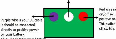
Red wire needs to run to an on/off switch and then to positive power on your battery. This switch is your fuel cut off switch.
