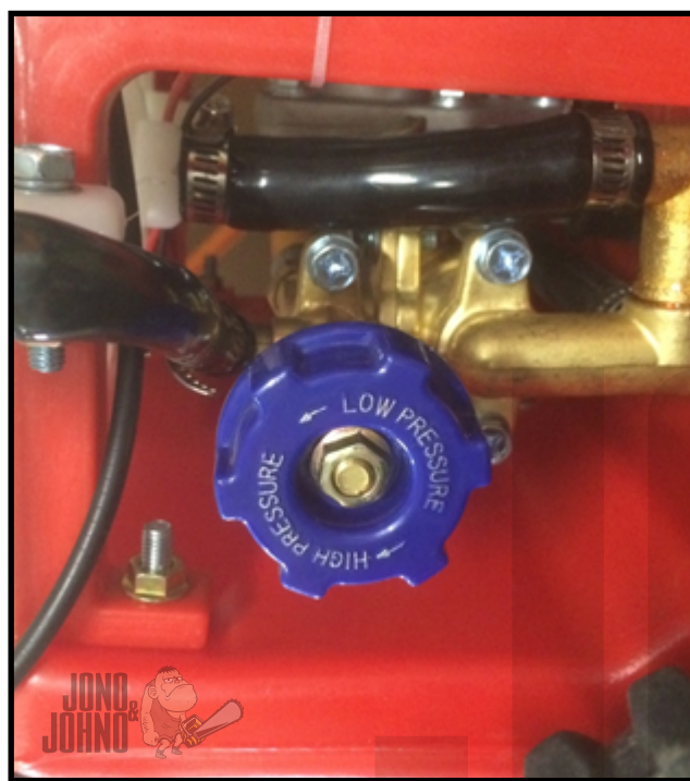
Pressure adjuster on pump
