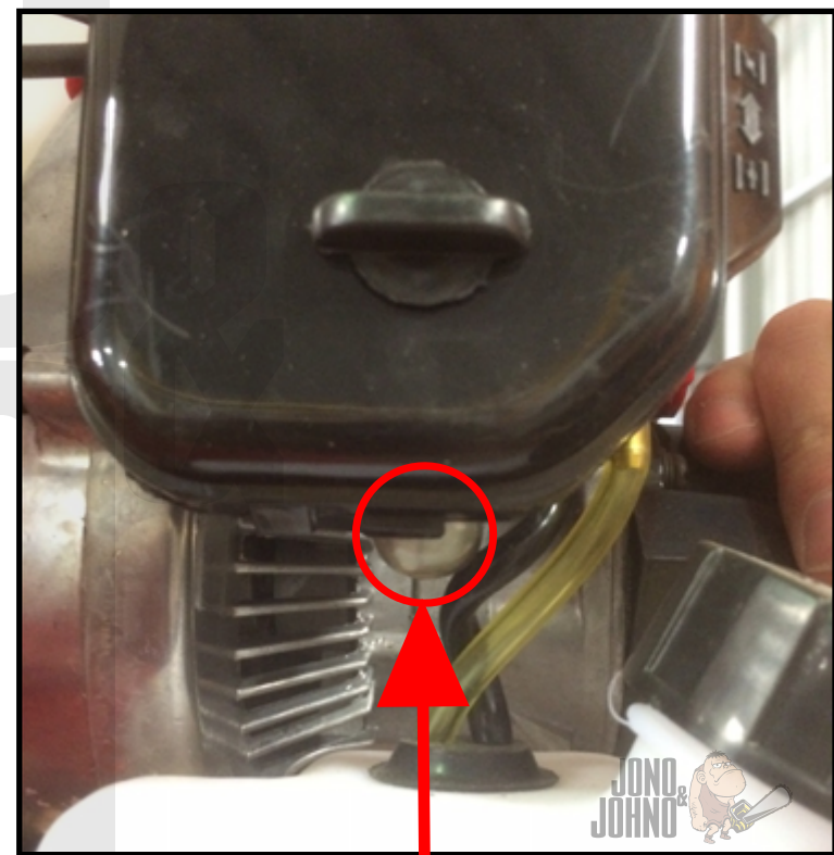
Fuel primer bulb. Pump this bulb before starting engine
