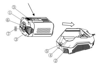
1.ZOMAX battery 2.ZOMAX charger 3.Release button 4.Red LED 5.Green LED 6.Battery power display button 7.Batterypower indicator
